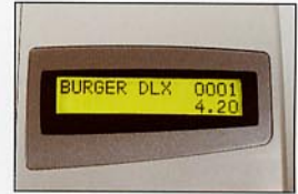
The 2-line alphanumeric backlit LCD display shows the item and price to minimize operator errors.
